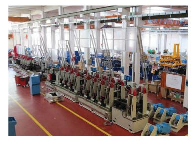
breakdown, finpass and sizing sections and the fully automatic coil strip loading system, which begins with a carousel with 4 arms of 30t each and a special car for automatic loading of each strip coil on the double decoiler.
