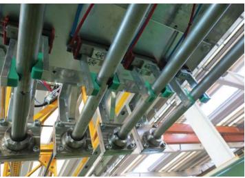
pneumatic arms for the tube feeding into a tool deburring device, to automatically remove both inside and outside burr.
