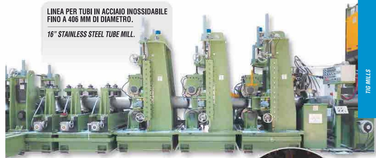
LINEA PER TUBI IN ACCIAIO INOSSIDABILE FINO A 406 MM DI DIAMETRO.
