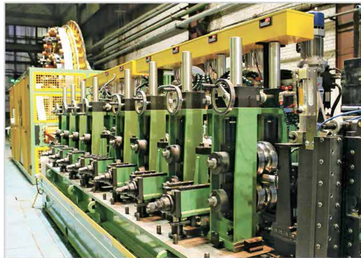
Complete line for the production of HF welded tubes in carbon steel with a size range from 18 mm to 76 mm O.D.
