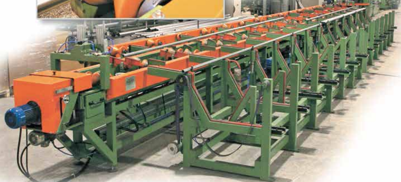
Tube unloading table with an incorporated automatic deburring system.
