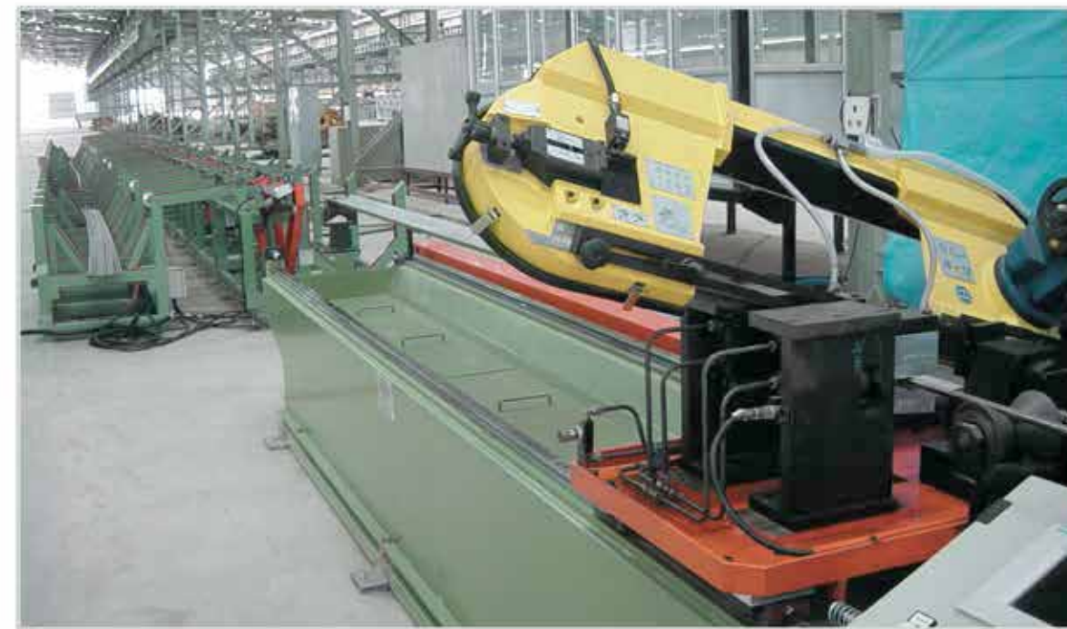
COLD SAW CUT-OFF MACHINE with the position of the cutting head at 45°. This cut-off machine is appropriate mostly to high speed production lines. It allows high precision and good tube end finishing.
