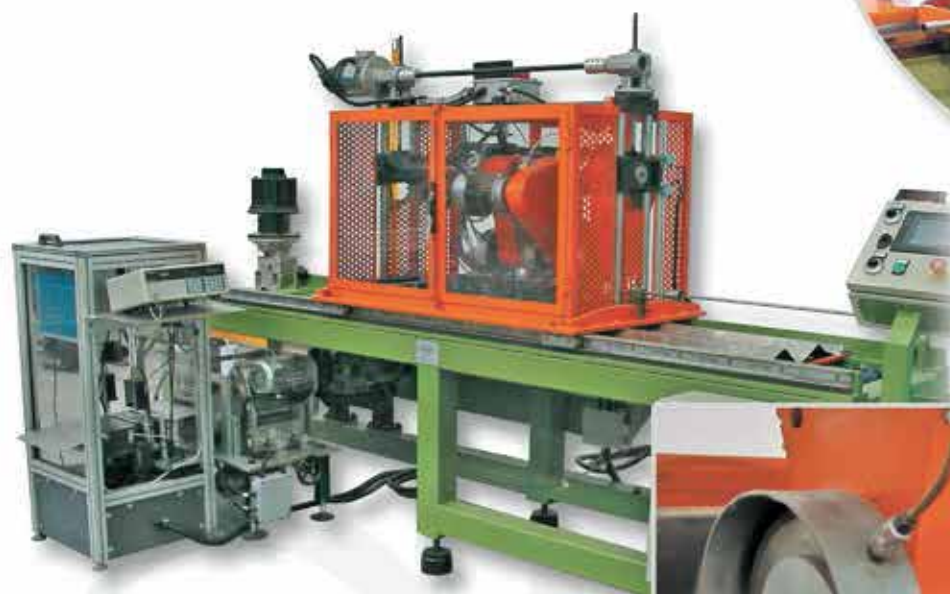
THREE-SAW CUTTING machine for small tubes complete with an automatic deburring unit.
